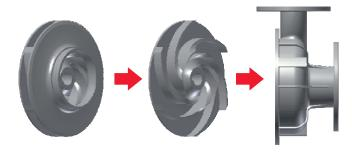
be used both for closed impeller (with wearing ring) and open impeller (with replaceable wearing plate): just with a few changes the pump can be adapted to new plant and process requirements. Pump casings are made by investment casting and they are electrochemically polished.
