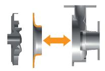
WEAR PLATE ALSO ON CLOSE-COUPLED PUMPS: Considering that the pump casing is the most expensive part in a close coupled centrifugal pump, the possibility to replace the wearing plate allows to reduce considerably maintenance and repairing costs.
